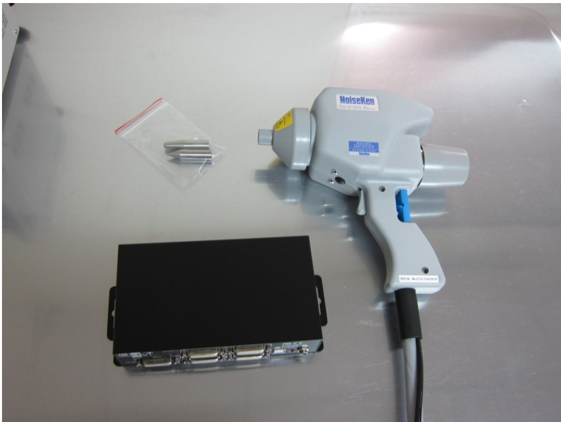
Picture 2: Discharge Gun and testing unit
