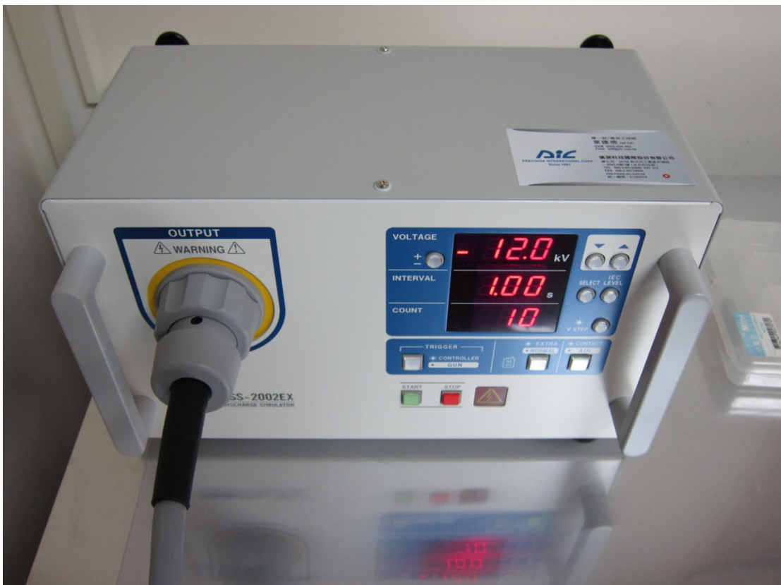
Picture 4: Adjust the voltage, interval and count for ESD testing
